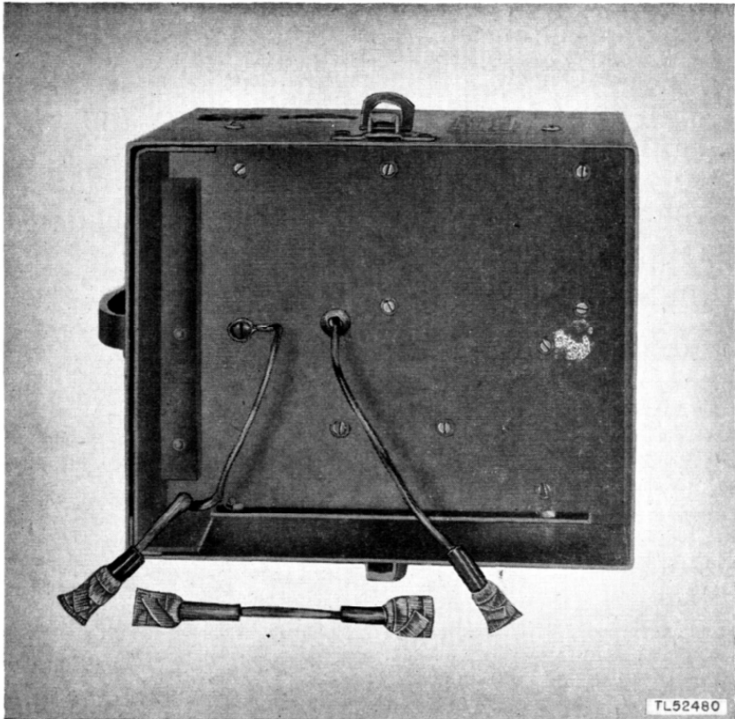
Figure 7. Converter M-222—battery compartment, battery connecting wires masked.
